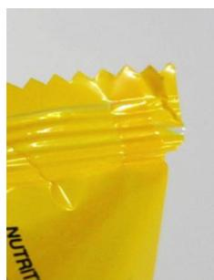
Figure 13: A serrated edge
