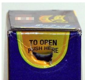
Figure 21: High force push tab
