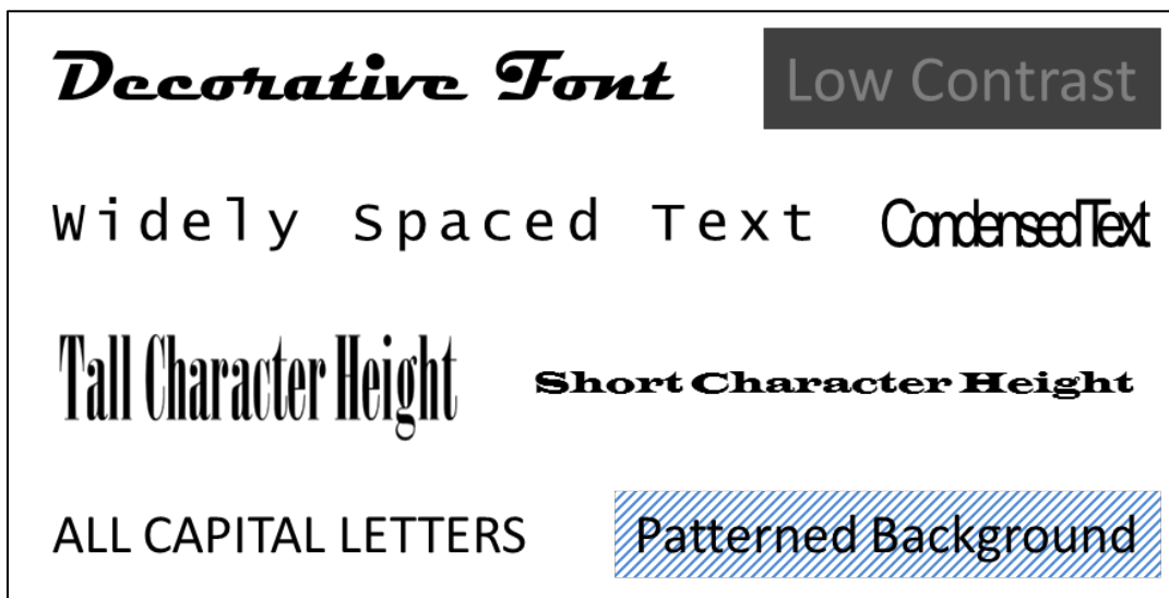
Figure 28: Examples of bad labeling.
