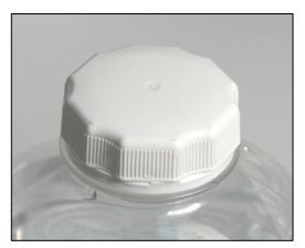
Figure 8: Cap with sharp edges.
