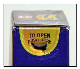
Figure 20: High force push tab.
