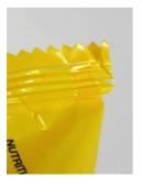
Figure 13: A serrated edge
